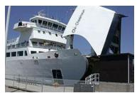
**Roll-on/roll-off** (**RORO** or **ro-ro**) ships are vessels designed to carry wheeled cargo such as automobiles, trucks, semi-trailer trucks, trailers or railroad cars that are driven on and off the ship on their own wheels. This is in contrast to lo-lo (lift-on/lift-off) vessels which use a crane to load and unload cargo.
