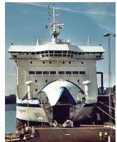
RoLo: A RoLo (roll-on lift-off) vessel is another hybrid vessel type with ramps serving vehicle decks but with other cargo decks accessible only by crane.
